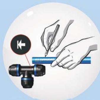
Mark the tube to indicate the insertion depth in the fitting (use the reference marks on the fittings or on the wrench).
