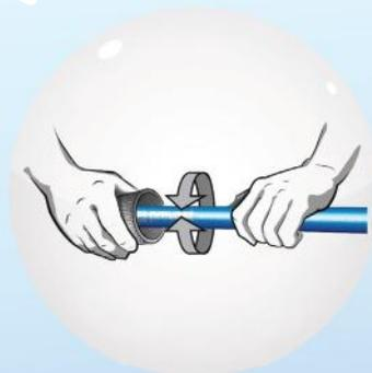
Chamfer the external edge of the pipe to make it easier to fit into the fitting and to avoid damage to the seal. A slight chamfer to the inner edge will eliminate any cutting residues. (For diameters 63 and 80 mm, use cutting and chamfering tool ref. PPS CTCHE6380).
