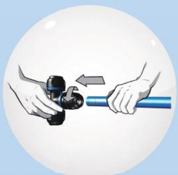
Unscrew the nut by several turns, and then insert the pipe while rotating it slightly until the recommended length is reached.
